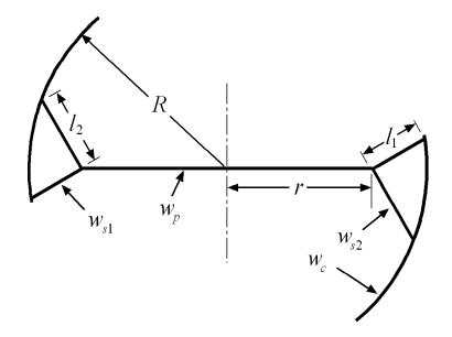
**Figure 1**. Plan view of the revolving elements of the 2-wing revolving door.
