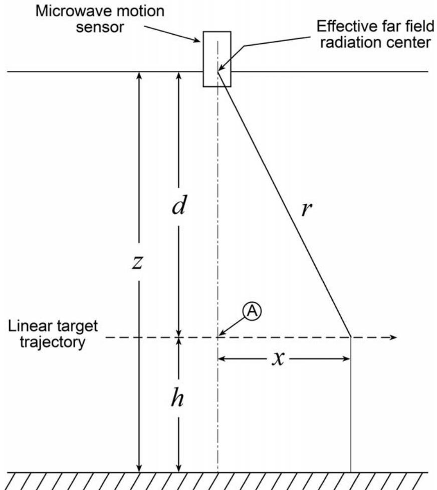
**Figure 1.** Relevant parameters in derivation of Doppler effect transition point along a horizontal linear trajectory.
