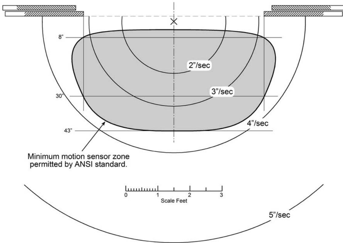
**Figure 3.** Minimum motion detection zone permitted by ANSI standard for sliding doors, with regions in which the Doppler effect for horizontal motion falls below the detection threshold of a microwave motion sensor.
